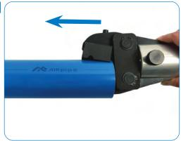
Manually open the jaws of the clamp and insert the aluminum pipe into the clamp as far as possible. 02
