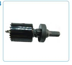
With the proper drill arbor & hole saw bit part numbers identified, thread the hole saw bit onto the drill arbor to create a single drill bit. 04
