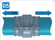
Pull the pipe back towards the outside of the clamshell to complete alignment.
