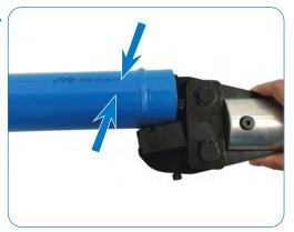
• Renew the operation until the required minimum number of lugs for each diameter is finished.
